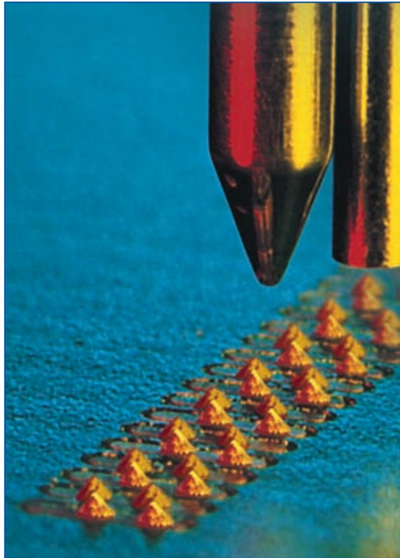
Microdispensing is the process of dispensing small volumes (less than 0.010-inch diameter) of solder paste and adhesives with consistent precision. Numerous factors must be considered in a microdispensing system, including platform, controlling software, syringe, dispensing needle and material feed pressure. However, the heart of any liquid dispenser is the pump, and equipment performance is typically
