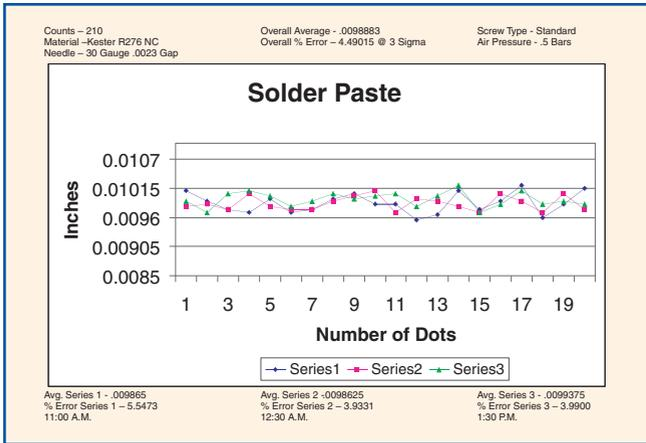
**FIGURE 2: Performance tests of dispensed solder paste with microvolume pump.**
