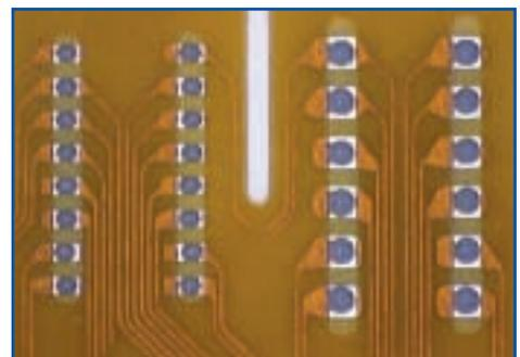
**Dispensing needles and pumps are required to dispense a variety of solder paste volumes. Dual pump configurations can be used to dispense two different dot sizes on the same substrate simultaneously.**
