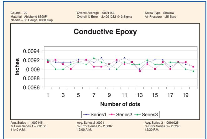
**FIGURE 3: Performance tests of dispensed adhesive with microvolume pump.**
