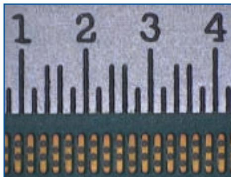
**Applications for CSPs and direct chip attach components require dispensed solder in volumes as small as 10 mils; the smallest increment in the scale shown above represents 0.02 in. or 508 µm.**
